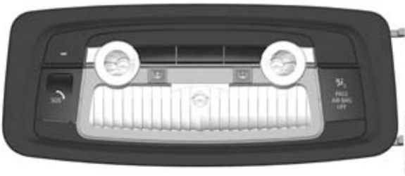
F12 Roof function center with indicator lamp for front passenger airbag deactivation
